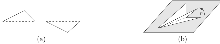
Figure 6: (a) In 2D, the same virtual link represents two configurations: a concave triangle and a convex triangle. (b) In 3D, the same virtual link represents many configurations with different dihedral angles \rho between the sub-chain's plane and its parent's plane.
