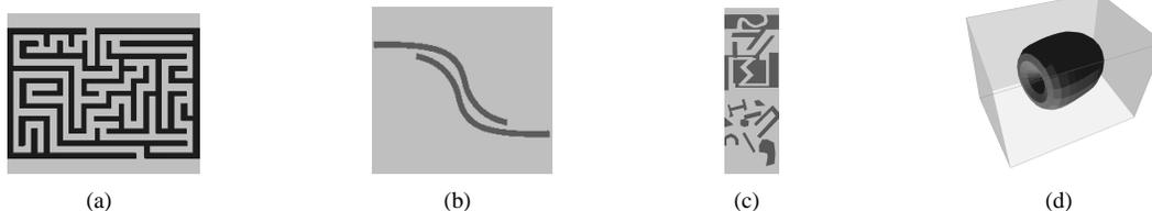
Fig. 9. Motion planning environments studied. (a) 2DMaze. The start and the goal reside at the two ends in the free space. (b) STunnel. The start and the goal are in the top left and the bottom right corners. (c) 2DHeterogeneous. The start is in the top free space and the goal is placed in the bottom cluttered region. (d) Bug Trap. The objective is to get out of the trap through the narrow passage.
