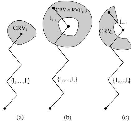
Fig. 4. (a)  $CRV_i$  is the constrained reachable volume of  $\{l_1, \dots, l_i\}$ . (b) The region that is reachable by the endpoint of link  $l_{i+1}$  is  $CRV_i \oplus \text{Reachable}(l_{i+1})$ . (c) The constrained reachable volume of the linkage  $\{l_1, \dots, l_{i+1}\}$  is therefore  $(CRV_i \oplus \text{Reachable}(l_{i+1})) \cap S_{i+1}$ .
