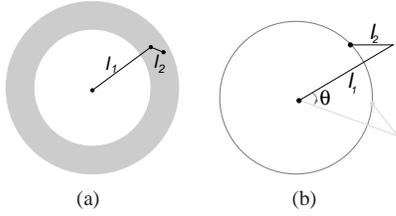
Fig. 3. (a) The reachable volume (gray region) of a 2 link chain robot,  $l_1$  rotates about the point in the center while  $l_2$  rotates about the endpoint of  $l_1$ . (b) If the end effector (black) can reach a point, then it can reach all other points that are the same distance from the base (gray circle).
